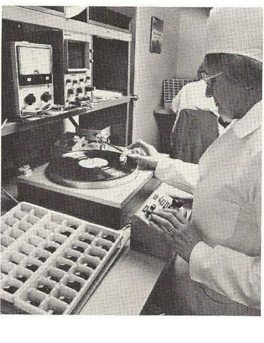
11. 100% quality control of all cartridges. All fully-assembled cartridges are individually played on a CBS STR-100 test record, monitored on a dual trace oscilloscope and measured with a VTVM.
