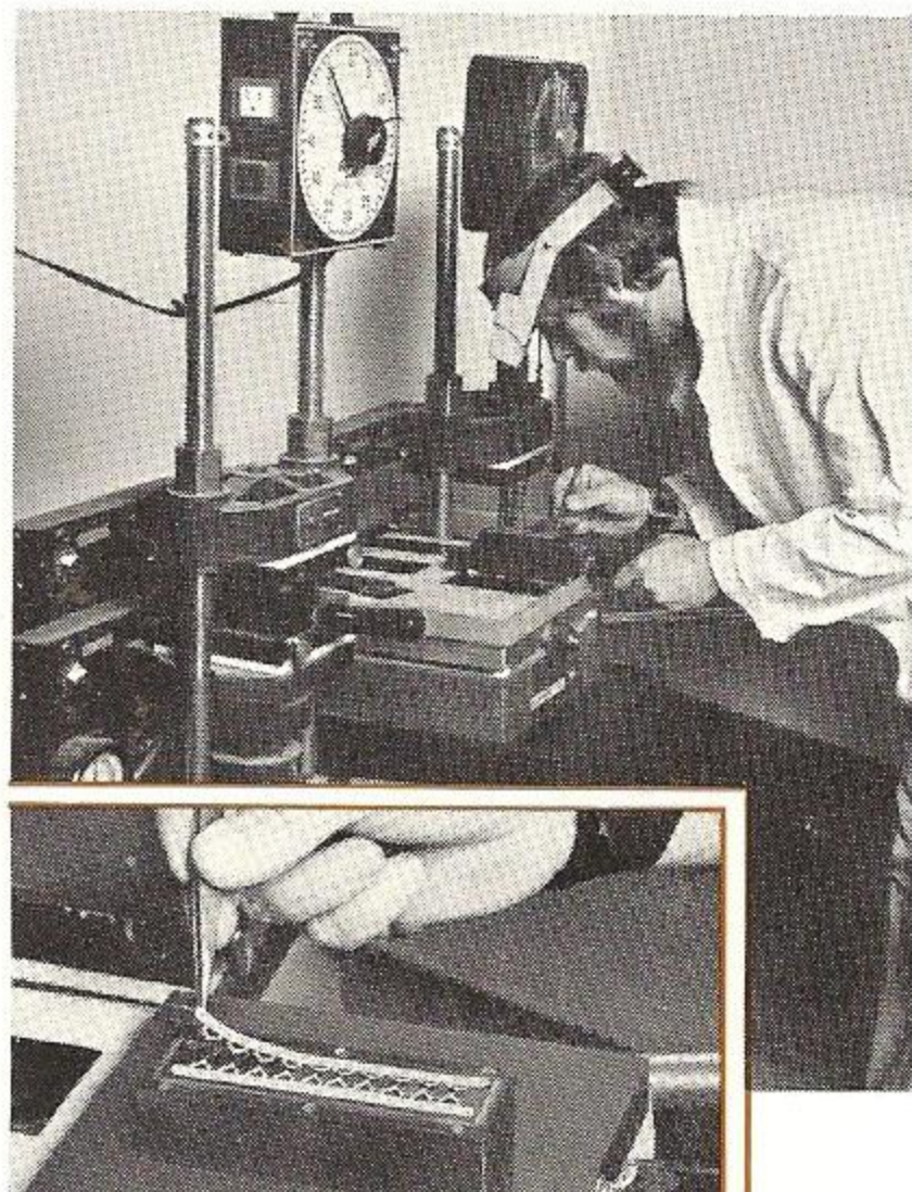
2. Rubber-molding press. Sixteen precision elastomers are employed in all Micro-Acoustics phono cartridges. Each part is individually molded; then inspected and tumbled in refrigerant to remove any excess "flash". The use of multiple elastomers provides greater long-term reliability and consistency than conventional single-bearing cartridge designs.
