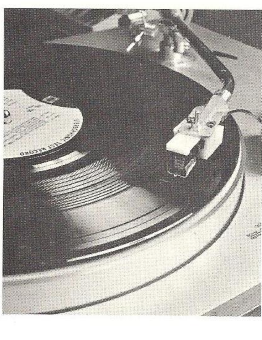
12. All areas of cartridge performance are tested. Tests include frequency response, channel separation, output level, tracking and transient ability. Only cartridges that fully meet published specifications are serialized and placed in stock for shipment.
